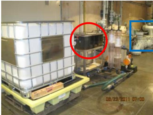
Flow is from left front to right rear in this photo. These inlet bioboxes (circled in red) receive system water just prior to the treatment injection location (boxed in blue in the rear/ right of the photo).
