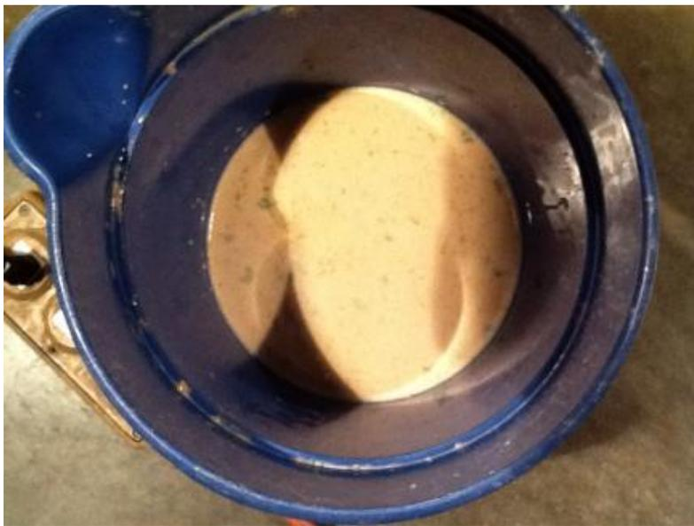
Figure 12. Microcystis algae (green clumps) in concentrated product solution of Zequanox in a bucket during the November 2011 treatment.
